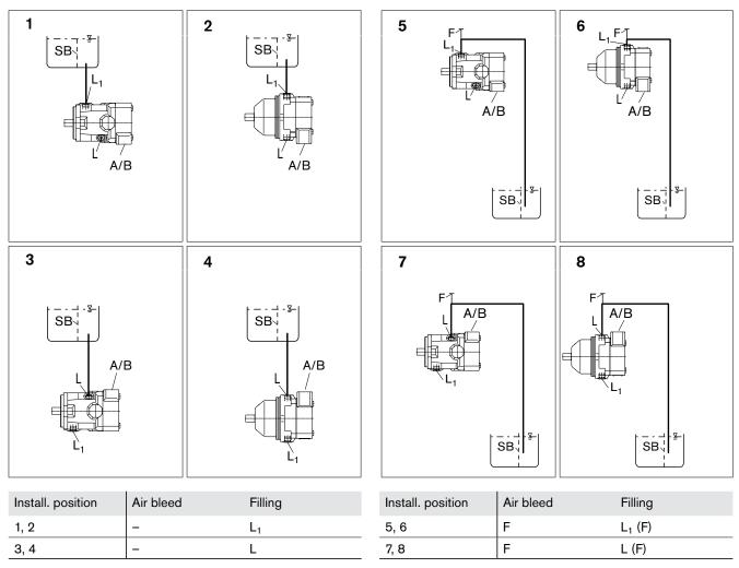
$L/L_1 = Case drain port$ , F = Air bleed resp. filling port, SB = Baffle.
